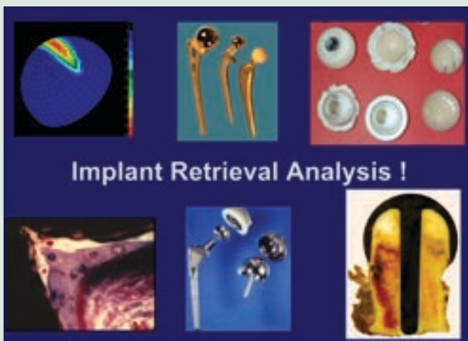
Figure 2. Retrieval analysis includes gross inspection, wear analysis, and histology.
